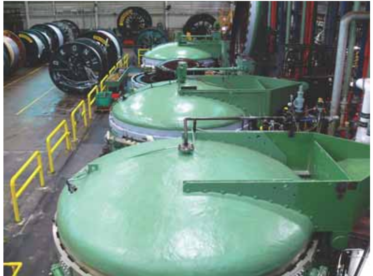
Four Vertical tanks for impregnating up to 345 kv HPFF cables in Lengths of 8,000 to 10,000 feet on 174" diameter reels.
