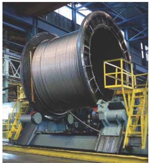
On right reel - Large 188" reel in the paper tapping machine.
