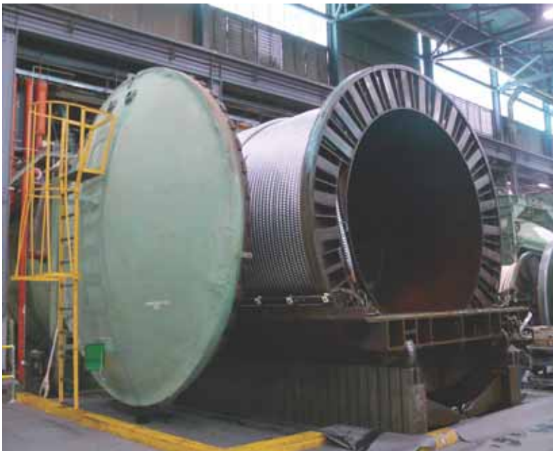
Horizontal Tank capable of impregnating up to 345 kv HPFF cables in lengths of 6,500 to 12,000 feet on 188" diameter reel.
